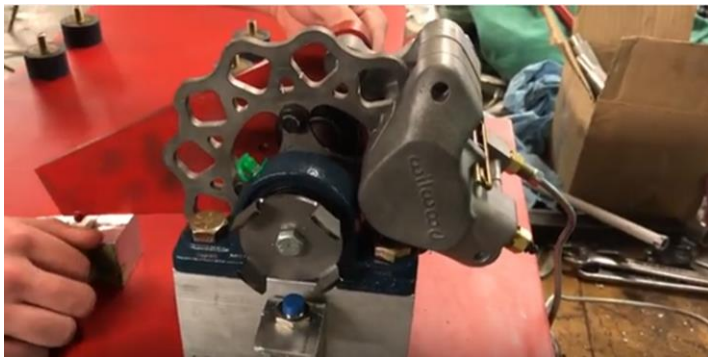
Figure 7: Side View of Proxy Sensor Mount, Brake Caliper, and Load Arm Layout [5].
